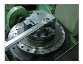
(29) Assemble main spool kit (33) into rear cover(32) after checking the direction to be correct.
