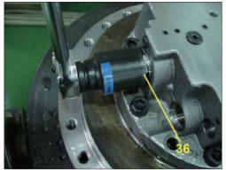
(31) Assemble relief valve assy (45) using torque wrench.
