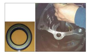
② Insert above shaft sub into casing (1) and assemble it with a jig.
