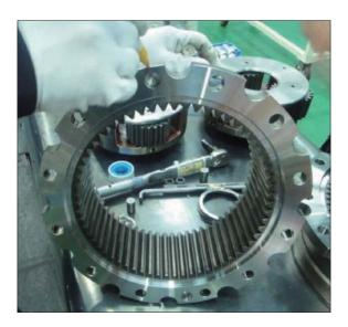
③ Align ring gear with pin parallel to put them into casing sub assy.
