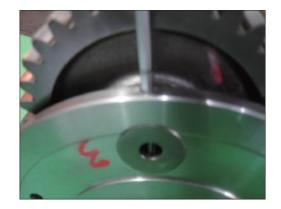
(5) Caulking both side of pressed spring pin 180° using caulking jig.
