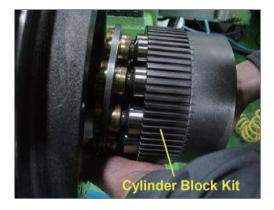
(22) Assemble separate plate (22), friction plate (21) into rotary block in regular sequence.Friction plate : 6 EASeparate plate : 7 EA
