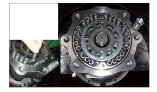
④ After hang valve casing (23) on hook, assemble it on casing (1) gently, then, tighten hex bolt (37, 38) tightly.
