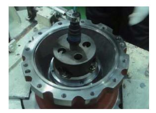
⑤ Align nut ring's bolt screw with lock plate's hole.
