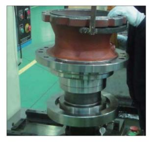
④ Remove oil seal & bearing taper (small) from casing.
