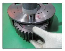
(4) Put spring pin into No.1 carrier using jig with force.
