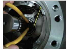
(16) Apply the grease to pivot (14)-2EA and then assemble pivot (14) into casing (1).
