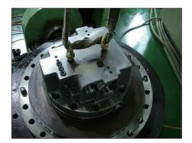
(5) Disassemble parking piston (23) using jig.
