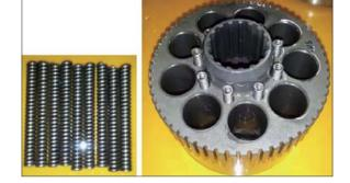
0 Put ball guide (10) on cylinder block (8).  $\cdot$  Ball guide  $\times$  1EA
