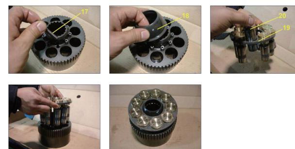
(21) Assemble rotary block kit into casing (1).
