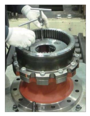
② Put No.2 sun gear into No.2 carrier sub assy.
