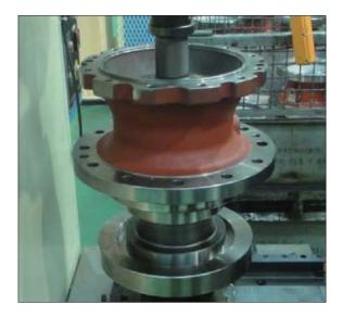
2 Assemble oil seal to casing.
