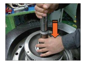
(14) Disassemble valve plate (36) from rear cover (32).
