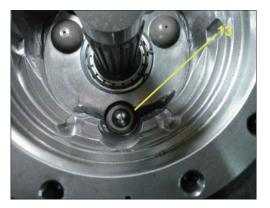
(19) Apply the grease to swash plate (15) and then assemble swash plate (15) into casing (1).
