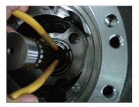
(13) In the casing (1), the arrow part of the shaft (8) using a rubber mallet taps and then disassemble the shaft (8) and roller bearing (9) to the other side.
