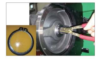
⑧ Disassemble shaft sub assy (3), oil seal(2), O-rings (18, 22) from casing (1).
