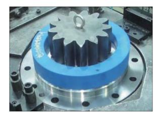
② Put drive shaft sub assy into casing.
