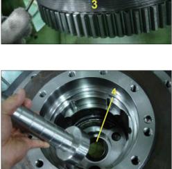
(15) Insert assembled shaft assy in the direction of the arrow into casing (1) using a rubber mallet.
