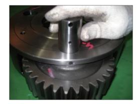
(3) Align spring pin with No.1 carrier spring pin hole and assemble spring pin accordingly.
