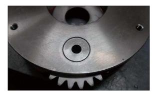
② After assembling No.2 needle bearing to No.2 planetary gear, put 2 pieces of No.2 thrust washer on both sides of bearing and install them to No.2 carrier.
