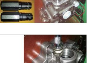
5 Disassemble plug (28), O-ring (29) from valve casing (23).
