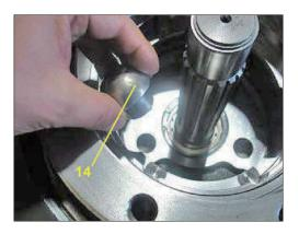
(12) Disassemble retainer ring (5) using pliers.
