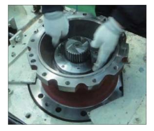
③ Remove drive shaft sub assy from casing.
