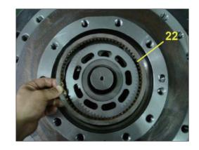
(24) Apply the grease to D-ring (24,25) and then assemble D-ring (24, 25) into parking piston (23)
