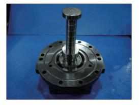
(7) Assemble spring pin (30), parallel pin (27) using small hammer.
