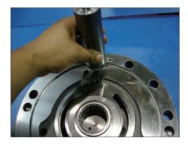
(8) Apply loctitle #242 on the restrictor (57, 58) and then assemble restrictor (57, 58), O-ring (43, 44) into rear cover (32).
