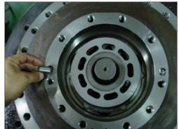
(23) Assemble parallel pin (31) into casing (1).
