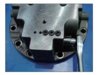
(6) Press needle bearing (10) into rear cover (32) using jig.
