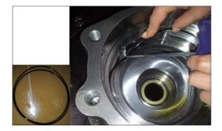
⑥ Insert cylinder block assy (8) into casing (1).
