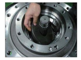
(10) Disassemble steel ball (13), swash piston (6)Hole in the casing (1) of two speed line is decomposed by injecting oil.
