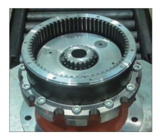
③ Removing No.2 sun gear from No.2 carrier sub assy. (Be sure maintaining it vertical with ground when disassembling No.2 sun gear.)
